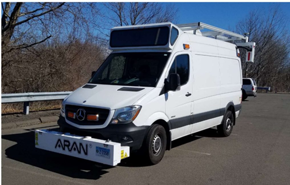
Figure 1-3 CTDOT Photolog Vehicle (One of Two Vehicles Currently Utilized)
